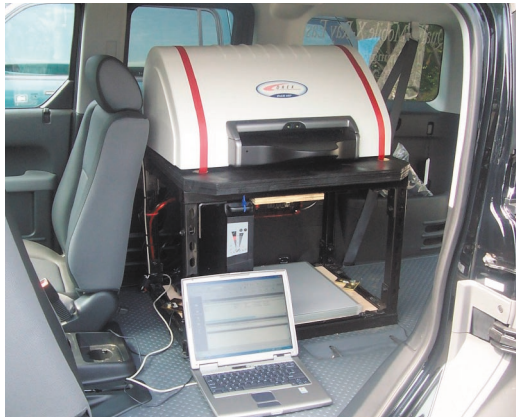
Orex CR images are sent wirelessly to the reading group — directly from the vehicle.
